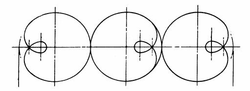
In the drawing (top of next page), broken line D-A-B is an arc of the circumference of the loop circle and is necessary in the layout before the painted tracing line is made. When the painted tracing is made, the arc is not painted on the two end circles; however, this arc is painted in on the center loop circle.
